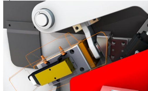
2 Fully automated locking of the rotor hood in connection with the fully automated opening of the rotor hood enables extremely short knife change times.
