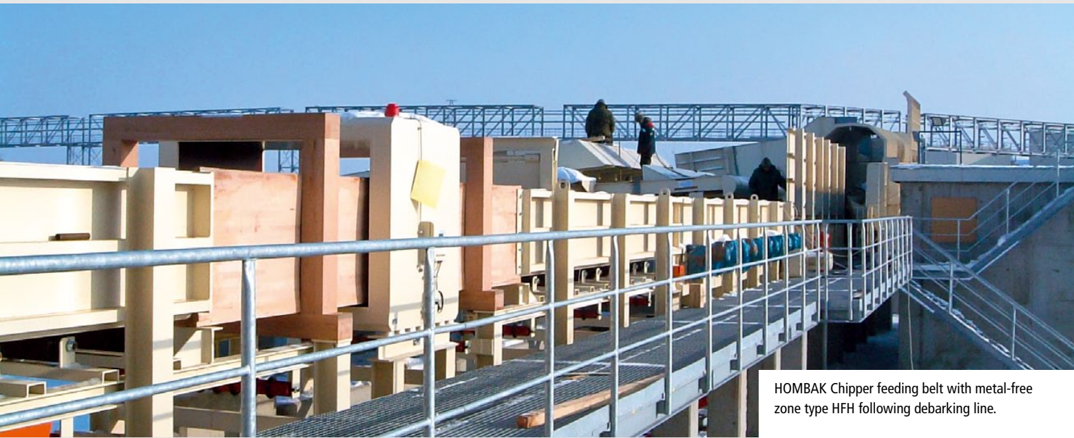
HOMBAK Feeding conveyor type HFA 6500 x 15000 with debarking line.
