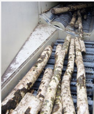
HOMBAK Rotor debarker discharge type HRA 1250 / 10
