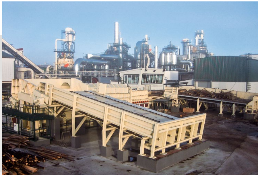
HOMBAK Feeding conveyor type HFA 6500 x 15000 with debarking line.
